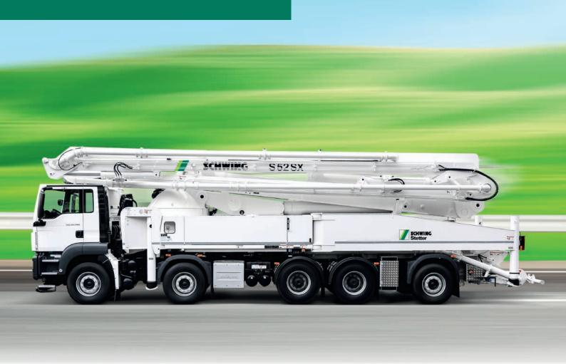
Vertical reach 52.00 m Concrete output max. 162 m³/h Pressure on concrete max. 85 bar
